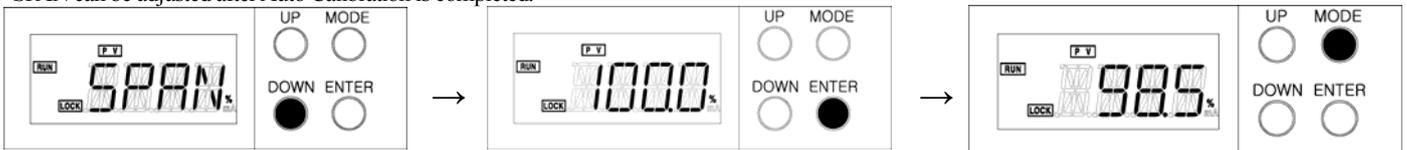
Push DOWN button for more than 5 seconds, and SPAN will be displayed.
